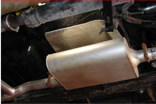
ZeroClearance® shields are an advanced patented alternative to traditional thermal and acoustical metal shields. ZeroClearance® shields are comprised of high-performance aluminum sheeting, a mechanically needle-punched fiber composite spacer, and a unique, high-temperature pressure-sensitive adhesive on the back for attachment.
