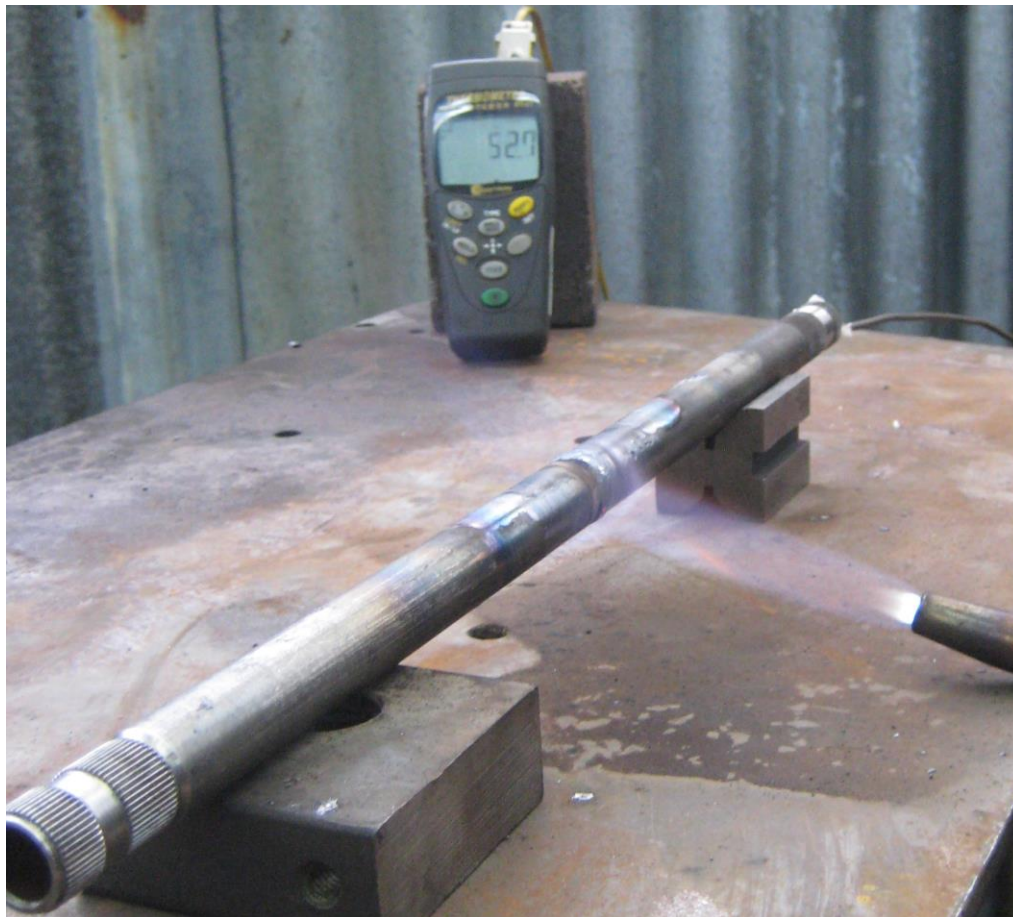
PWHT in progress, with thermocouple inserted in centre of spigot.
