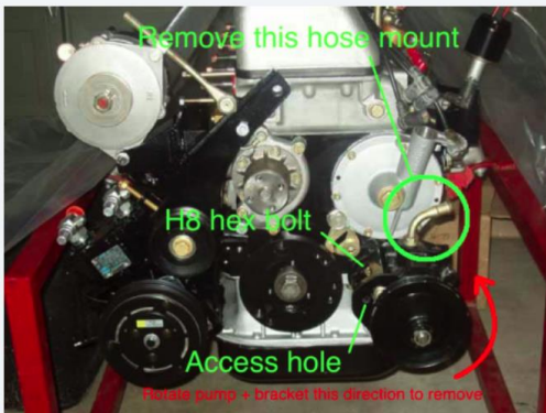
280sl power steering pump + bracket removal.jpg (605.67 kB, 800x600 - viewed 219 times.)
