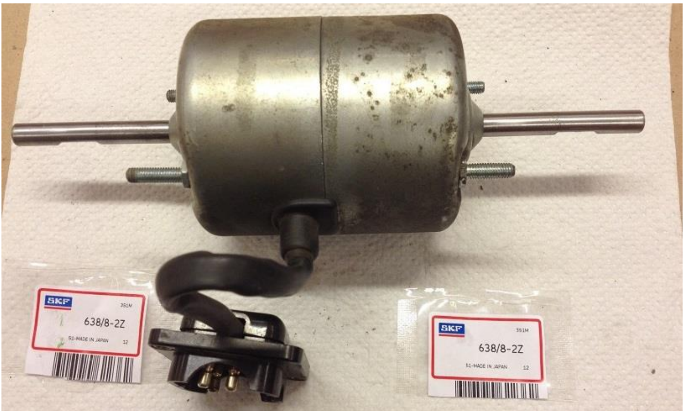
ready to install fan motor - running total of quieter and with a little more speed / air flow.
