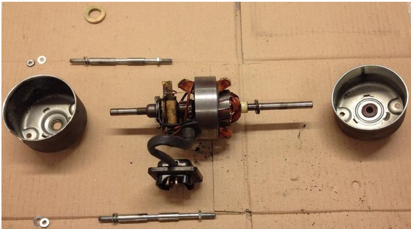
Dismantled housing halves
