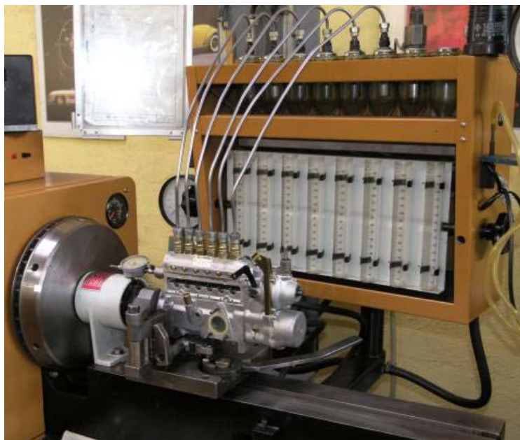
A six-ram pump with vacuum control on the pump test bench.
