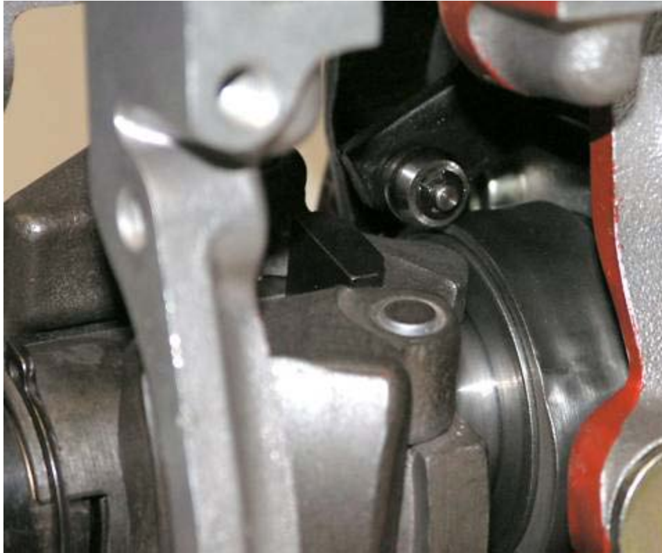
View into the innards: The feeler roller (above) takes the information from the space cam.
