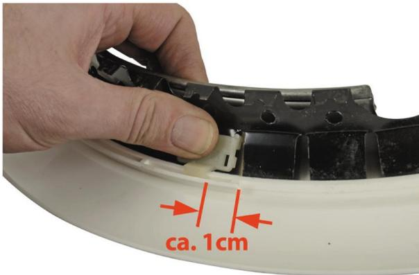
3) The remaining 5 clips are mounted, spreaded regularly, at the stainless steel rim.
