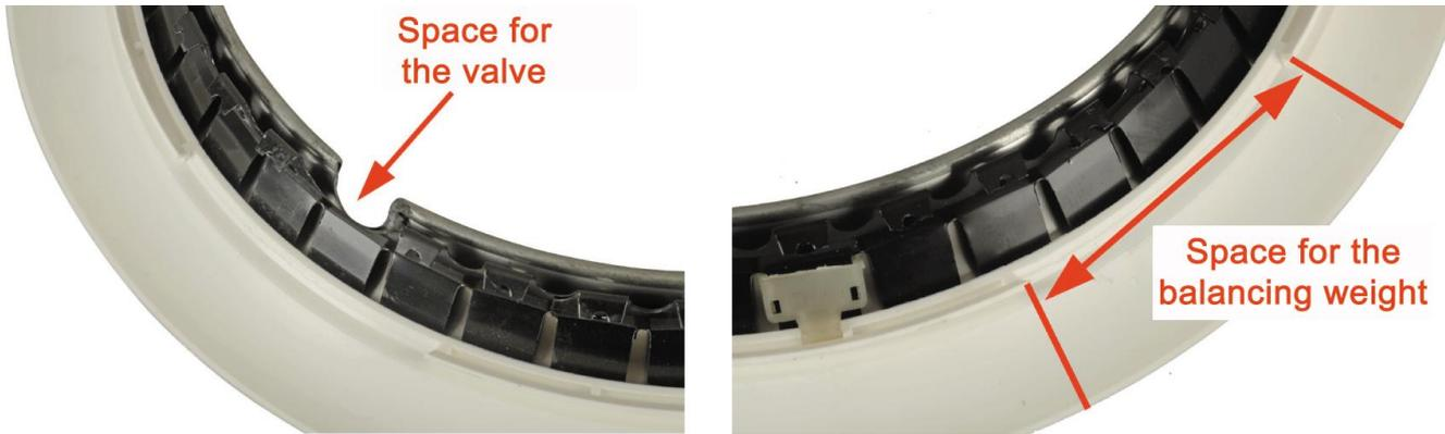
2) The first clip has to be positioned directly beside the space at the sidewall ring with a distance of 1 cm. To do that, put the “nose” into the notch of the sidewall ring and clip it into a sheet metal of the stainless steel ring.
