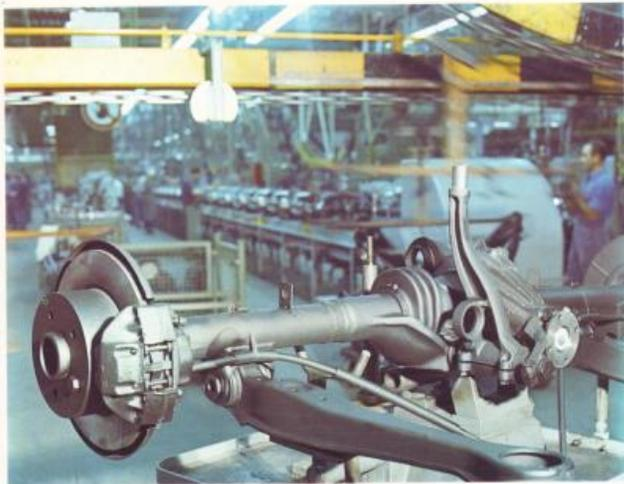
The Mercedes-Benz single-joint swing axle, with compensating spring, gives the 280 SL its famous road holding qualities, which make fast driving safe.
