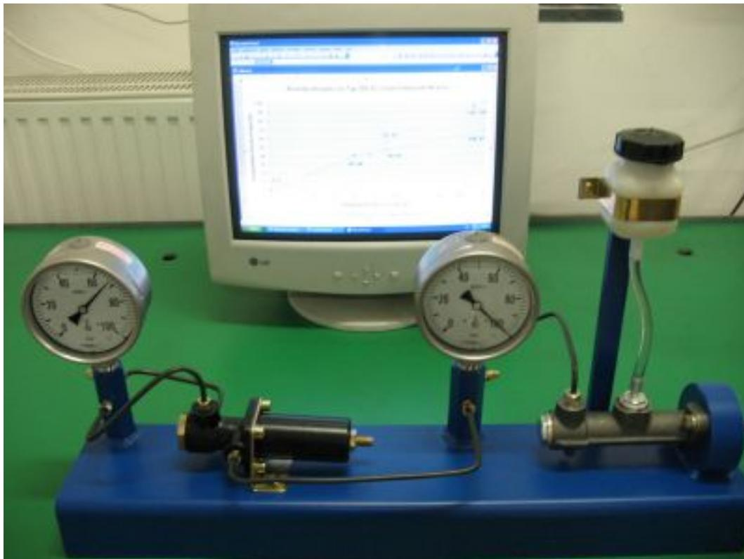
The test must also be done at an entry pressure of 100 bars. In this case the value of the exit pressure should be  $67 \pm 3$  bars, which is
