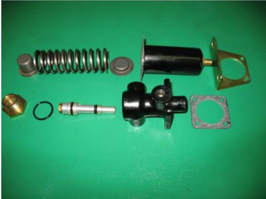
In the photo you can see the renewed parts of the disassembled brake pressure regulator of a Type 250SL. Since repairing this component was forbidden, it has never been possible to purchase parts for it. Believe it or not, the smaller rubber sleeve that can be seen on the piston is today produced by a little Hungarian
