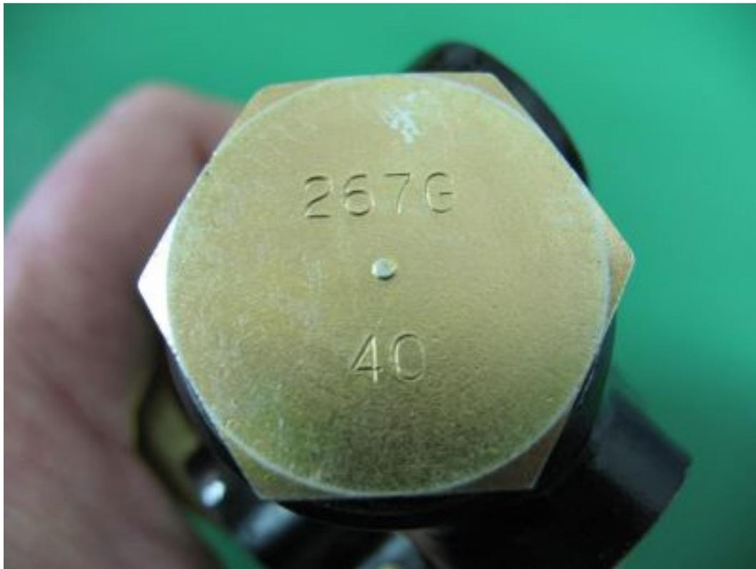
The number '40' punched into the plug screw means that the previously mentioned switch point of the brake pressure regulator is around 40 bars. The assembled brake pressure regulator will be tested on a test bench that was manufactured by us.
