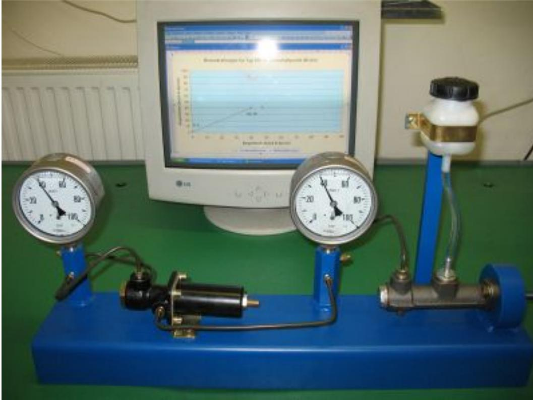
It can be seen that the pressure entering the front- and the rear-wheel brakes increases at the same rate up to 40 bars. We enter the measurements into a little program (that we developed) which displays the performance graph of the brake pressure regulator.
